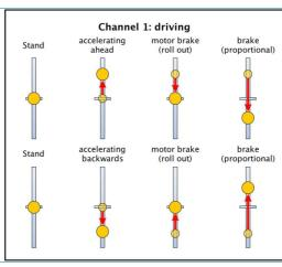
To switch off the motor, proceed as follows: stop the vehicle for at least three seconds. After that the throttle stick must be put to the bottom and released back quickly to the center position. This procedure may not last longer than one second.
